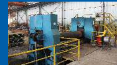
数显上辊万能式卷板机 Digital display on roller universal machine
