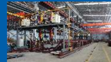
H型钢龙门式自动埋弧焊机 H type steel Longmen type welding machine
